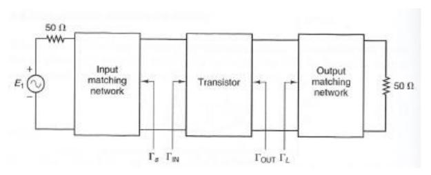
A conjugate match using transducer gain would require simultaneous adjustment of both input and output matching networks because changing one changes the other.
